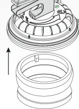
Remove the handle by sliding it backwards. Do not press hand lever.
